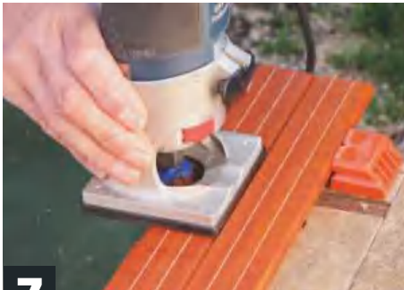
7 Add decorative chamfers on both inside and outside edges. Use a bearing-guided chamfer bit in a palm router or table mounted
